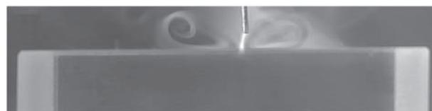
Fig. 4 Flow pattern induced by the plasma flow in the air near the water surface.
