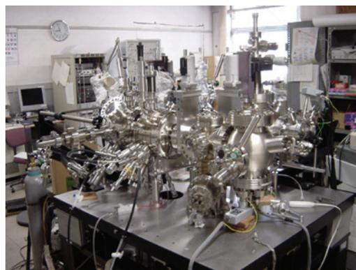
Fig.1 A photograph of the sample preparation and analysis chambers on active vibration isolation system.
