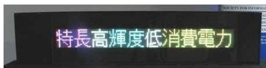
Fig. 7. Character display panel with CNT cathode.
