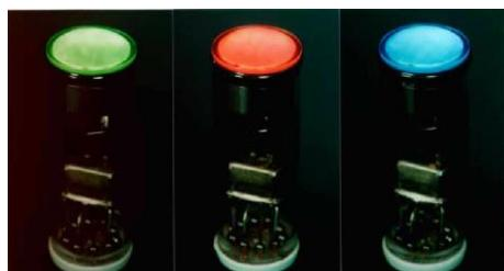
Fig. 6. Vacuum fluorescence display (VFD) with CNT cold emitter.
